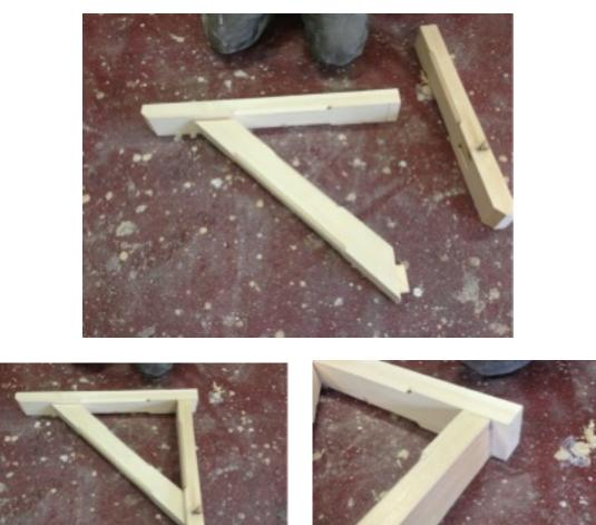
• Dry fit all the joints together to make sure the bracket will go together
